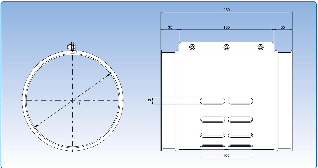
Durchmesser:  $\varnothing 80 - \varnothing 200$  mm.
